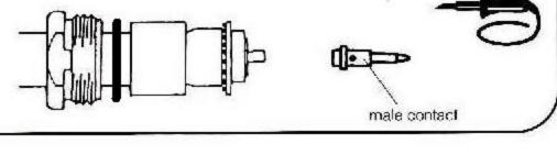
Slide plain gasket and clamp nut up to ferrule trapping braid. Fit front insulator over contact to butt against rear insulator and press sub-assembly into body as far as possible.
