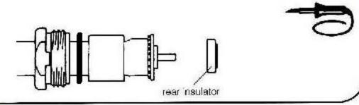
5 Fit contact (male for plugs, female for jacks) onto centre conductor. Hold cable and contact tightly together and solder.
