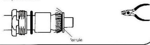
3 Trim back dielectric and check the length of the protruding centre conductor.
