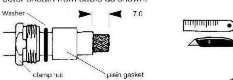
Pold back braid and push ferrule over dielectric to trap braid between outer sheath and ferrule. Trim off surplus braid.
