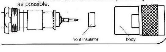
7 Engage and tighten clamp nut.
