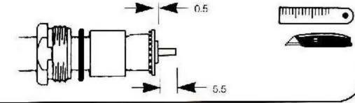
Tin centre conductor, then slide rear insulator over dielectric to butt against ferrule.
